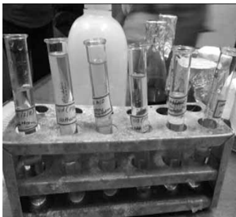
Figure 2 Moringa leaves oil extracted by Oil extractor with Acetone , Alcohol, Methanol ,Pet ether, Chloroform, n-Hexane and with aqua extract.
